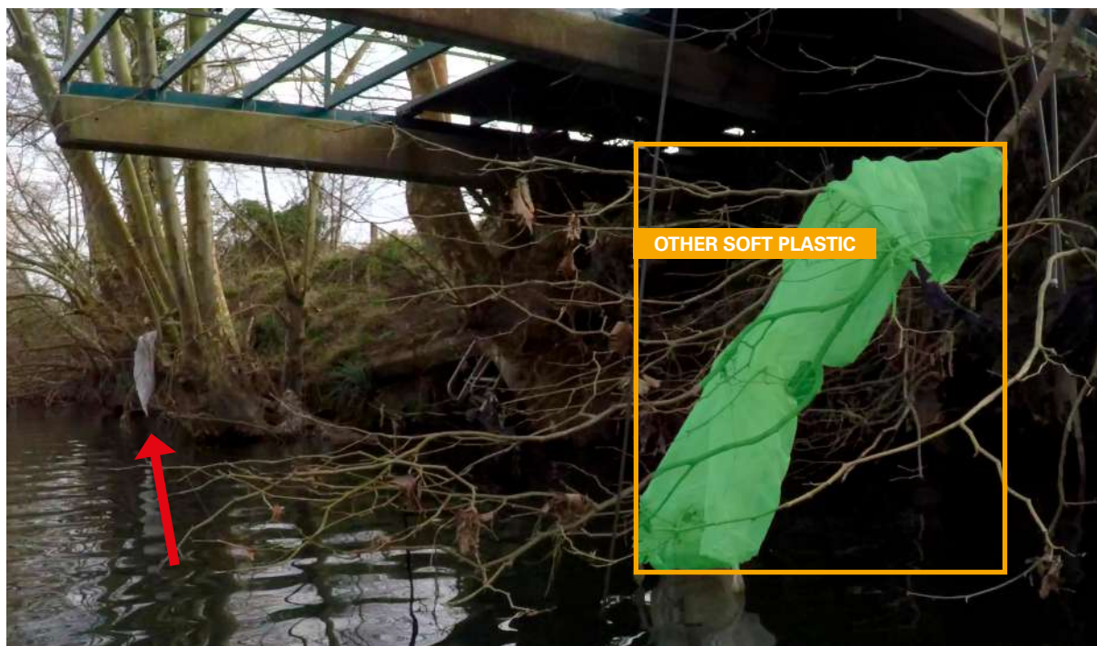
Figure 23 | Above | Example of image with error: the largest piece of plastic is detected, but the small one to its left is not.
